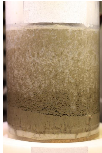
Figure 6 Specimen during freezing test after 4 days
